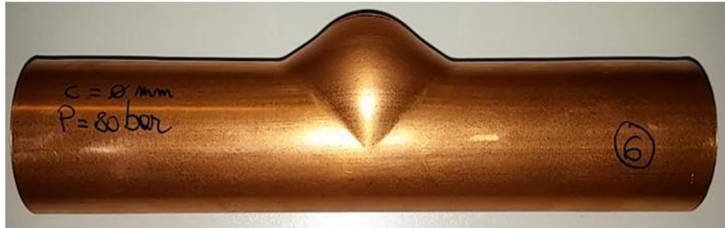
Breakage due to insufficient axial feeding
