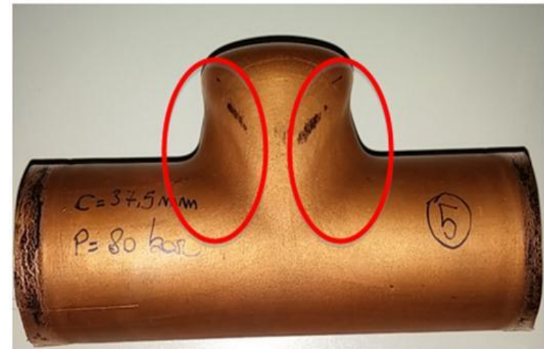
Insufficient filling due to insufficient pressure
