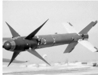
Figure 2. (a) A titanium guidance section housing for a (b) Sidewinder missile.
