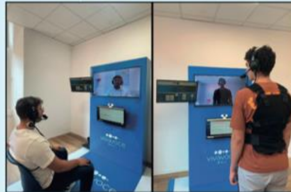
Figure 1. The figure illustrates some of the equipment used for AMFS. The left image shows a participant with microphone and headphones during a fluency assessment session. The right image shows a participant during a rehabilitation session in the post-intensive phase, which includes auditory (microphone + headphones), visual (monitor), and vibrotactile (vest) stimulation. The figure shows some pieces of the equipment in this study and is protecting a patient (patient number: 100200002002), under Patient and Tackles Office, (© UniV & Muscarà, 2024).
